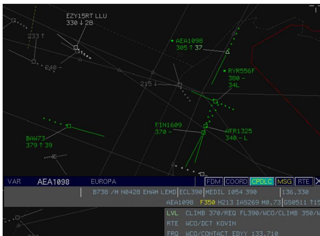
Figure 8: Controller Pilot Data Link Communications at Maastricht UAC. Picture courtesy of Eurocontrol.
