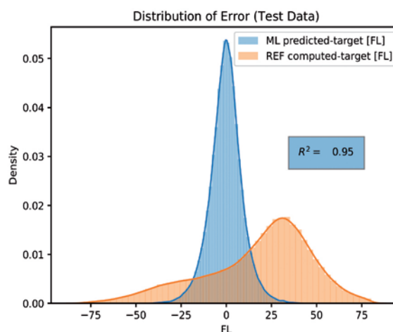
Figure 2: Distribution of Error concerning climb phase prediction. AI based methods proved to be more accurate than conventional methods to predict climb behavior of individual flights.
